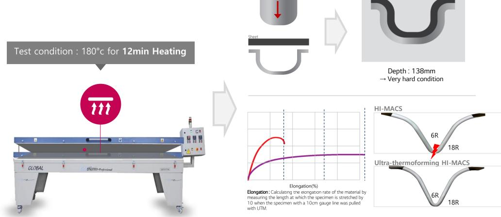
The elongation rate of the 'Ultra-thermoforming HI-MACS' is more than 3 times better than that of existing HI-MACS.
