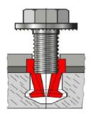
a) Insert the sleeve in the hole and drill the screw in the sleeve
