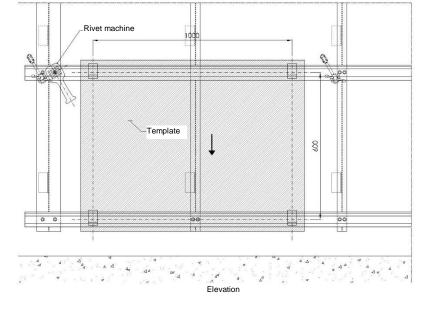
② Lock the template on the starting rail and following rails. Check the position of the following rails. Adjust if required. Install the based starting rail permanently with fixed.
