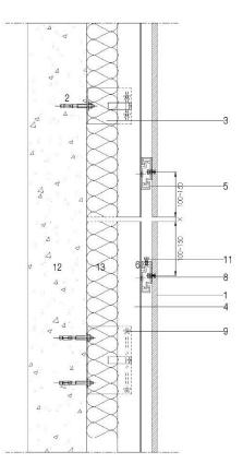
Figure 25 - Splitting the framework: Aluminium uprights of length  $\leq$  3 m
