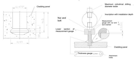
Geometry of Keil cladding drill bit
