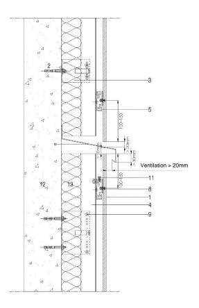
Figure 26 - Splitting the framework: Aluminium posts between 3m and 6m in length
