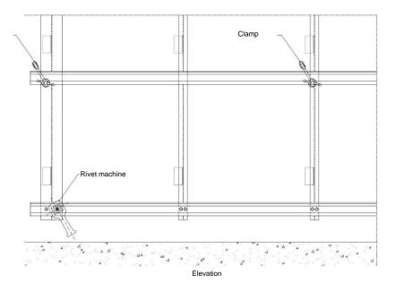
$\fbox{1}$  Install the level starting rail permanently with rivets. Install the following rails by temporarily using the clamps.
