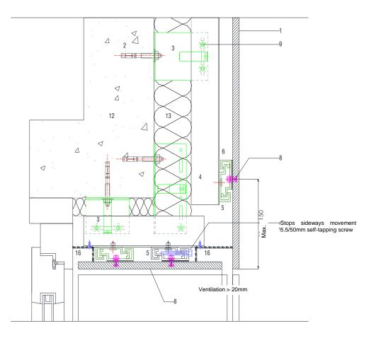
Figure 20 - Window lintel with HI-MACS<sup>®</sup> panel cladding
