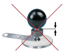
You cannot push the gauge down to the base section with the thickness wedge.
