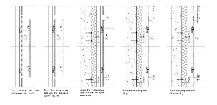
Figure 27 - Replacing a component
