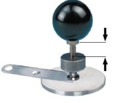
2 - Place the thickness wedge between the panel and base section of the control gauge. The machined hole is compliant if you cannot push the gauge down to the base sec-
