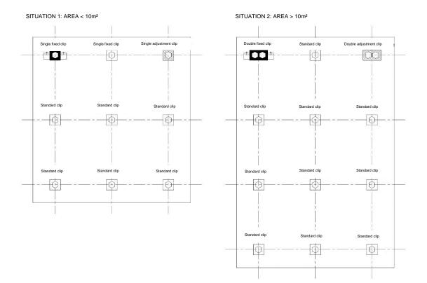
Figure 7 - Positioning clip types
