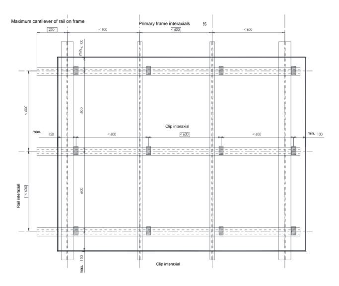
Figure 9 - Clip and frame interaxial distances
