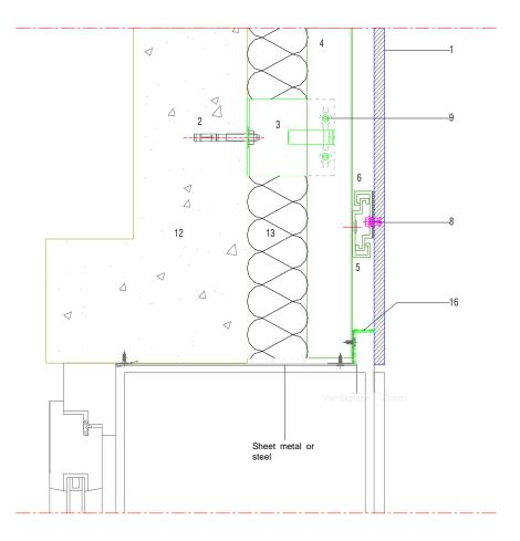
Figure 19 - Window lintel with sheet metal cladding
