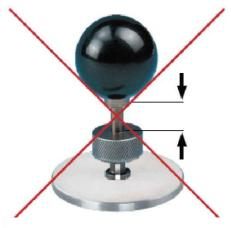
You cannot push the gauge down to the base section without the thickness wedge.
